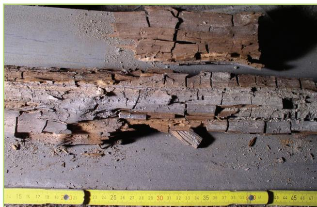
Figure 1. Example of untreated wood with "dry rot".
